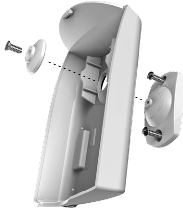
FIG 2. Installation of the Standard Swivel Bracket.
