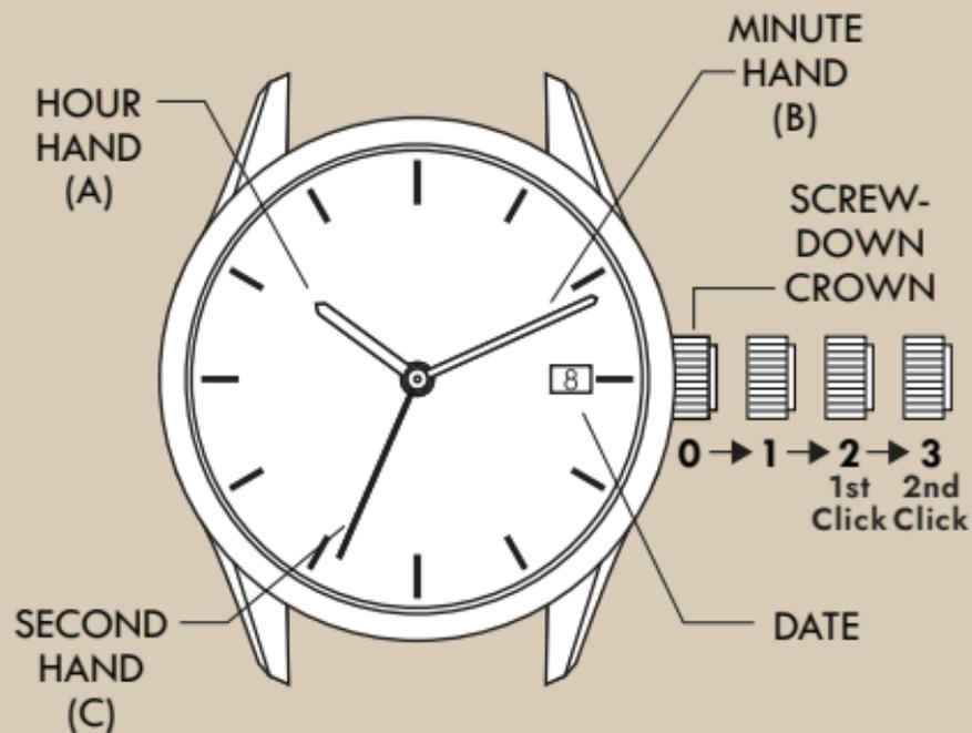
If your watch has a screw down crown feature, release the watch from the screw down position.
