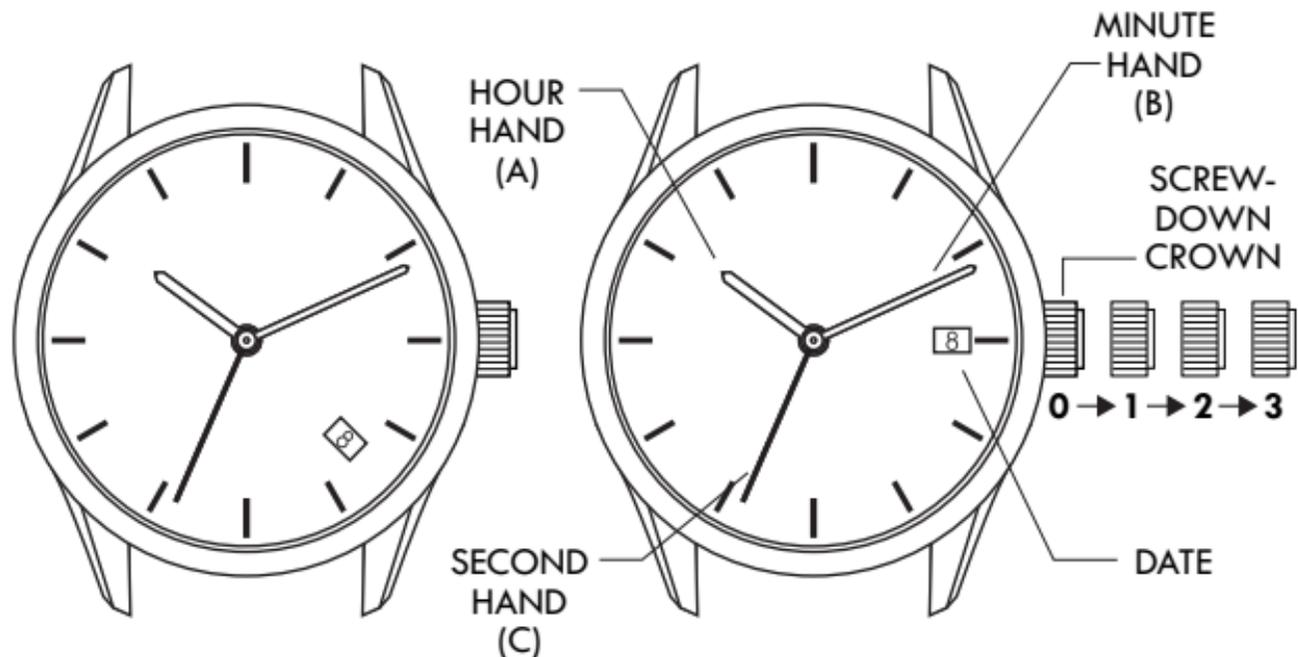
**If your watch has a screw down crown feature, release the watch from the screw down position.**
