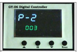
We already preset it to 003 before shipment. That is to say, if your setting temperature is 200°C, it will slow down the heating speed when it heats up to 197°C for a safe purpose.
