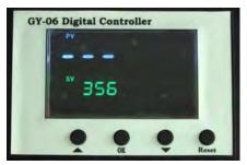
Press button, the temp light is on. Select with arrows the temperature according to different transfer material (Normally 180 ~200 )
