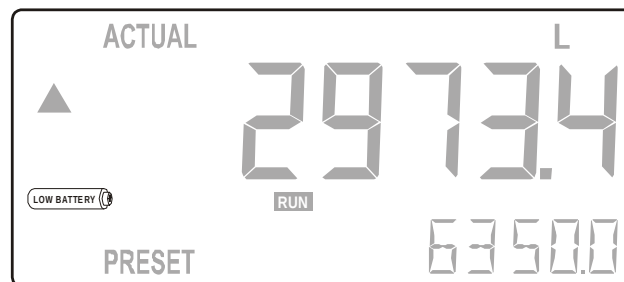
Fig. 6: Example of low-battery alarm.
