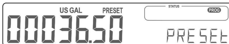
Figure 5: Example display information during programming preset value.
