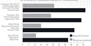
Slip Resistance Test EN ISO 13287:2012, performed by TUV Rheinland LGA Products GmbH in Leipzig, Germany during August 2010\* On a scale where 0.0 is the absence of friction and 1.0 is very high friction (e.g. dry carpet), SFC rated .63 – more than tripling the .18 minimum standard. All SFC shoes use the Shoes For Crews patented slip-resistant outsole. Product tested:BRIDGETOWN 28740
