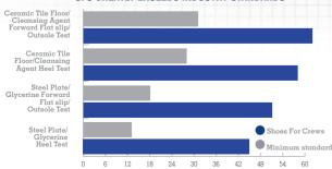
Slip Resistance Test EN ISO 13287:2012, performed by TUV Rheinland LGA Products GmbH in Leipzig, Germany during August 2018\* On a scale where 0.0 is the absence of friction and 1.0 is very high riction (e.g. dry carpet), SFC rated. 8.3 – more than tripling the .18 minimum standard. All SFC shoes use the Shoes For Crews patented slip-resistant outsole. Product tested:SRIDGETOWN 28740
