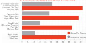
Slip Resistance Test EN ISO 13287:2012, performed by TUV Rheinland LGA Products GmbH in Leipzig, Germany during August 2018\* On a scale where 0.0 is the absence of friction and 1.0 is very high riction (e.g. dry carpet), SFC rated. 63 – more than tripling the .18 minimum standard. All SFC shoes use the Shoes For Crews patented slip-resistant outsole. Product tested: BRIDGETOWN 28740
