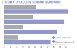
Slip Resistance Test EN ISO 13287:2012, performed by TUV Rheinland LGA Products GmbH in Leipzig, Germany during August 2018\* On a scale where 0.0 is the absence of friction and 1.0 is very high friction (e.g. dry carpet), SFC rated .63 – more than tripling the .18 minimum standard. All SFC shoes use the Shoes For Crews patented slip-resistant outsole. Product tested: BRIDGETOWN 28740
