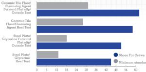
Slip Resistance Test EN ISO 13287:2012, performed by TUV Rheinland LGA Products GmbH in Leipzig, Germany during August 2016\* On a scale where 0.0 is the absence of friction and 1.0 is very high riction (e.g. dry carpet), SFC rated. 6.3 — more than tripling the 1.8 minimum standard. All SFC shoes use the Shoes For Crews patented slip-resistant outsole. Product tested:BRIDGETOWI28740
