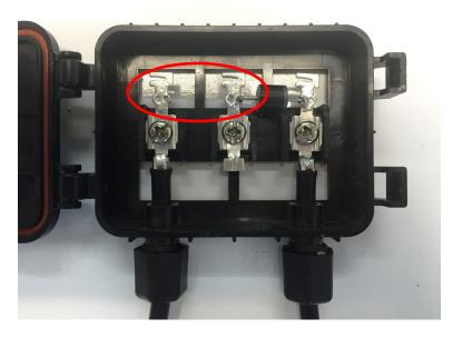
4. If the leads on the replacement diode are not bent into a "U" shape, pre-bend the leads in the same manner as the diode that was removed in Step 2. This can be done easily with a pair of pliers or by hand.
