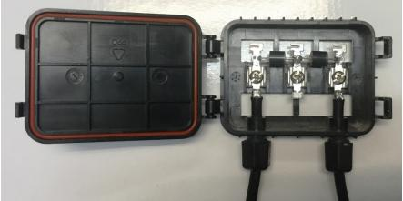
2. Remove the diode that requires replacement from the terminals by using the tip of the solder iron under the lead of the diode and prying or lifting each lead of the diode separately.
