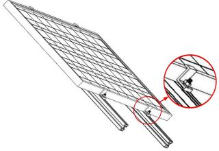
17. Set the tilt angle by moving the Adjustable Angle L-Brackets (Item 4) within the T-Slot Bracket.
