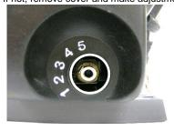
8 By losening screw(2) the cover can be moved slightly up, down and left, right
