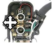
9 Repeate steps 6, 7 and 8 until the stem is successfully centered. Tighten the outer cover screws(step 3) and then the dial set (step 2)
