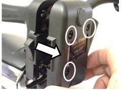
4 Remove screws(2) on each side of the *thermal fuse* and replace
