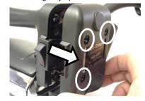
4 Remove *power switch* from the body, then from the terminals
