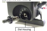
3 Remove screws(3) from the *outer* cover and gently open it
