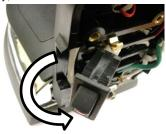
5 Place the new *power switch* with the light indicator facing down
