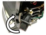
Once installed in place, push-in power switch to eliminate open gaps
