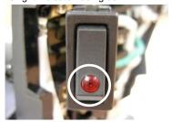
6 Install *power switch* starting from the terminals, then the body
