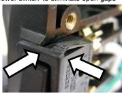
8 Inspect all prongs are making contact on each terminal
