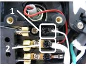
**5** Pull and Remove the wire insulator
