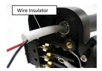
6 Remove *tip screw* and gently then the *microswitch* assembly along with wires
