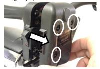
4 Remove screws(2) from terminal 1 and 2
