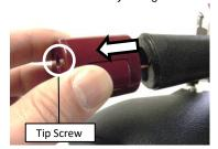
Install the new *microswitch assembly* starting from the wires
