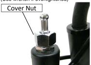
2 Remove cover nut and fitting off the solenoid valve
