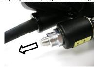
4 After removal of *plunger* and *spring* make sure the valve is empty inside
