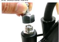
Tilt iron to the side and gently waggle, the *plunger* and *spring* will start sliding out
