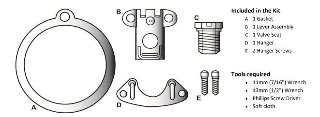
David<sup>™</sup> Bucket Steam Trap Repair Kit RK-890 is an inexpensive way to repair your existing steam trap that is not working properly or leaking. Over long period of use, the bucket trap's seat and the free floating valve lever gets worn out and won't operate propelry to open and close the steam trap. The repair kit will fix your malfunctioning steam trap by replacing all intenal parts with no need to remove your exisiting steam trap from the pipe line. Made of stainless steel (SUS304).
