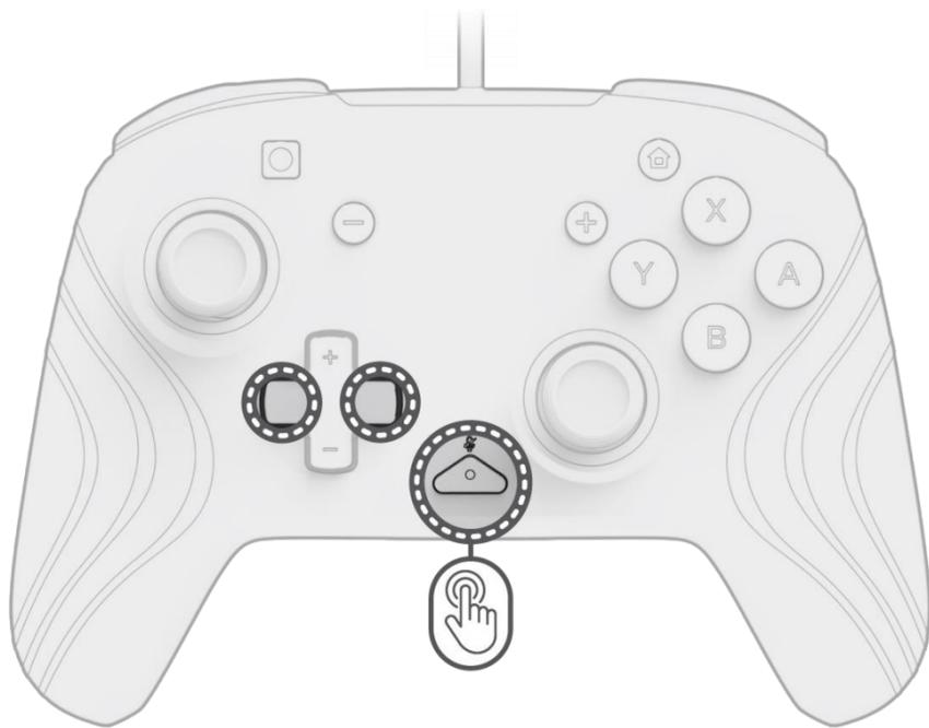
A. Hold down the “function” button and use the Left/Right button on the D-pad to change the LED’s color.
