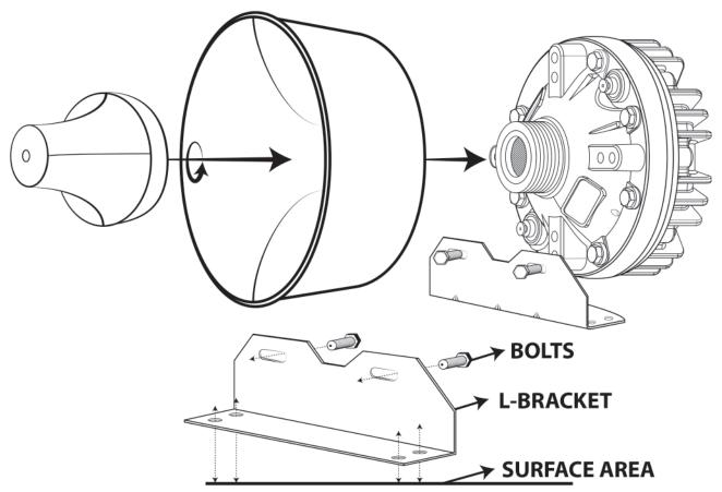
UTILIZING BOLTS LARGER THAN 0.25", SECURE THE L-BRACKET TO THE SURFACE MOUNT.
