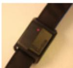
The red light indicates RE-vibe is charging. (During regular use, a flashing red light indicates battery is low.)
