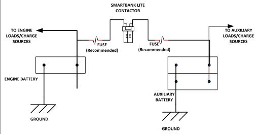
CAUTION & WARNING!: Under sizing the cabling between the batteries and split charge contactor will cause overheating and possible damage to the contactor. Extreme overheating may lead to fire.
