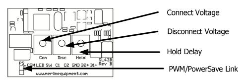
"Con" is Connect Voltage, "Disc" is Disconnect Voltage. "Hold" for the Hold Delay timer.
