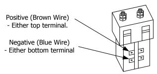
CAUTION: Incorrect wiring of the contactor will burn a track on the SmartBank Lite PCB and render the unit un-operational. This is not covered under warranty. The top connector tabs are connected together, therefore, wiring the positive and negative to the top two (or bottom two) terminals will cause a direct short circuit across the PCB.
