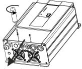
Access the connection compartment by removing the two screws and sliding the red cover downwards.
