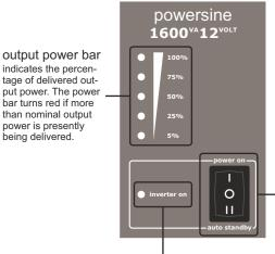
StandBy (ASB) mode. See chapter 3 for more details on the ASB mode "inverter on" or "error" indicator
