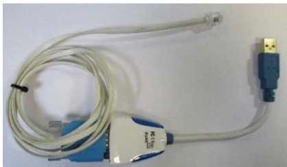
Fig 1: FTDI Converter and Serial Cable
