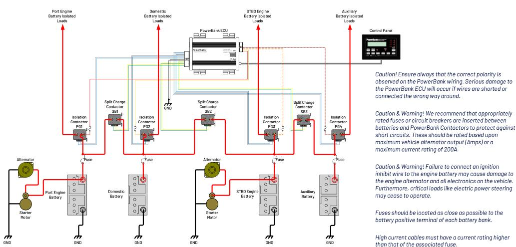
The above diagram shows a typical 4 Battery Bank example installed on a twin-engine boat using a PowerBank control panel.
