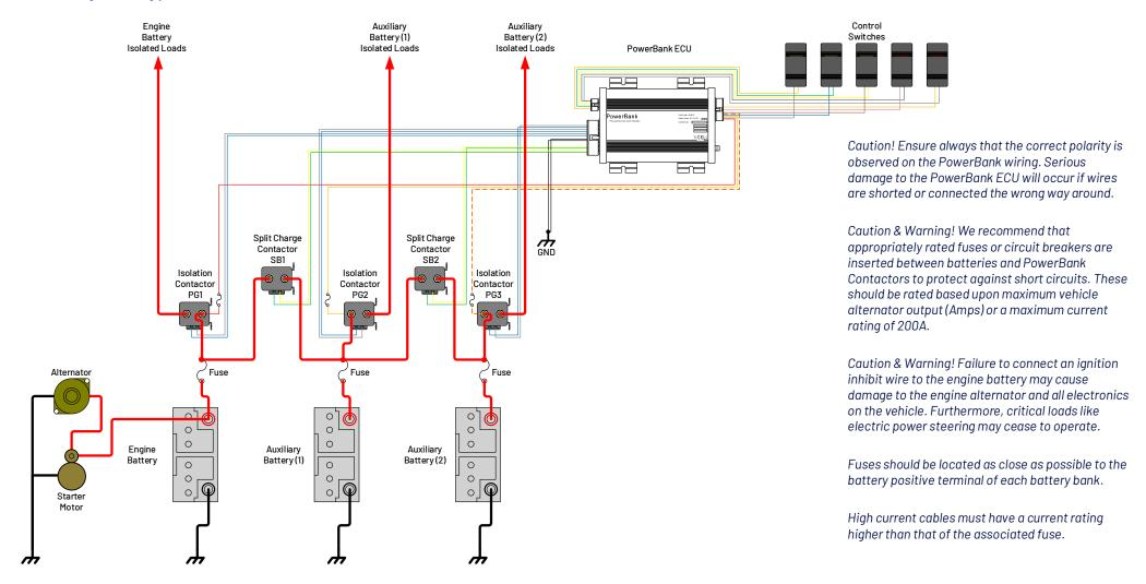
The above diagram shows a typical 3 Battery Bank example installed on a vehicle using control switches with internal LEDs for status indication.
