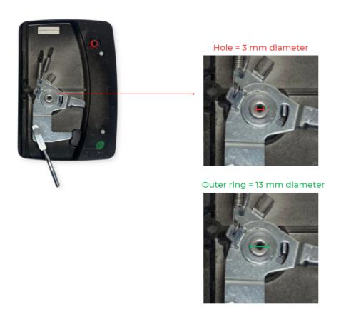
3.) Check that the plate / bolt portion on the back of the interior latch look exactly like the example below:
