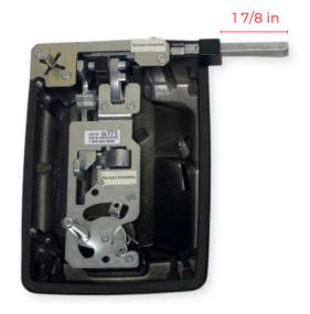
2.) The hole on the back of the interior latch measures 3 mm in diameter. The outer ring measures about 13 mm in diameter. If the hole on your latch is much larger than this, your latch may have been recalled - please contact your motorhome manufacturer for a replacement.
