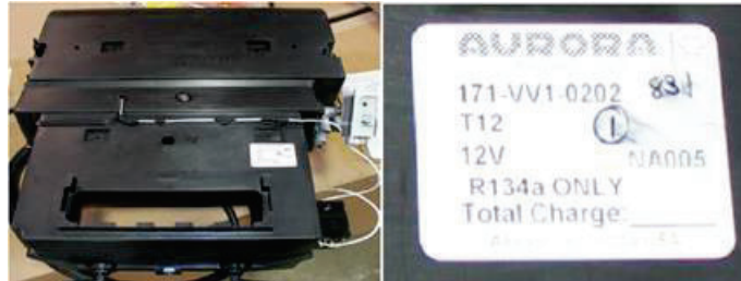
Figure 1: Aurora HVAC Unit Label example.
