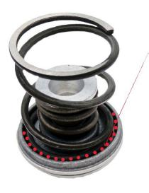
Ensure the tapered part of the spring is located in this part of the servo cover. Fitment should be recessed.
