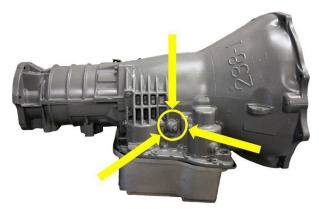
If pressures are too high or low, adjust the pressure regulator screw on driver side of the valve body with a cut down 3/16" allen key.
