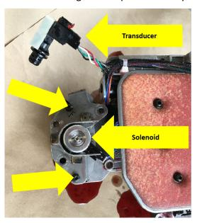
Insert the transducer into the opening.
