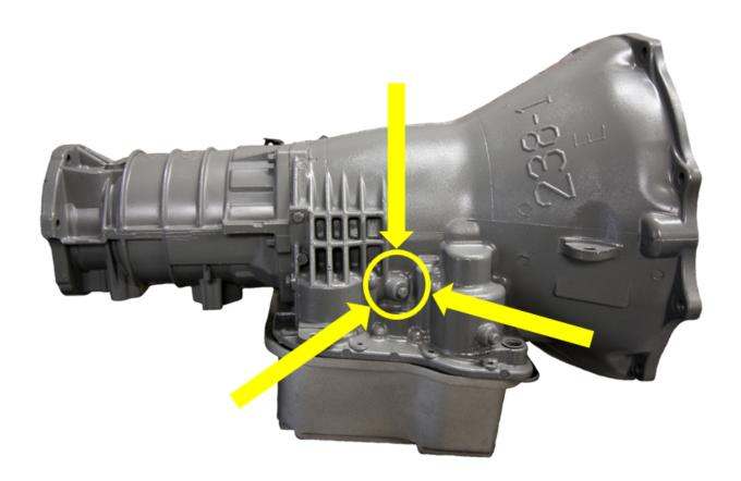
If pressures are too high or low, adjust the pressure regulator screw on driver side of the valve body with a cut down 3/16" allen key.
