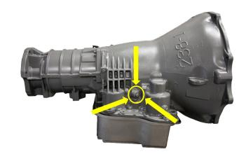
\*\* Before verifying WOT pressure, ensure there is some line pressure rise when throttle position is increased. If idle pressures are 75-90PSI, and transmission has been cycled through gears 1-4 on jack stands, double check fluid level running in neutral. Check WOT pressures, ONLY after verifying fluid is full, via road test in a safe, controlled environment
