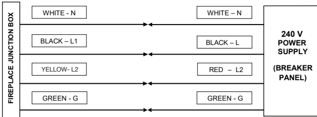
Figure 8 240 V Hardwire Installation
