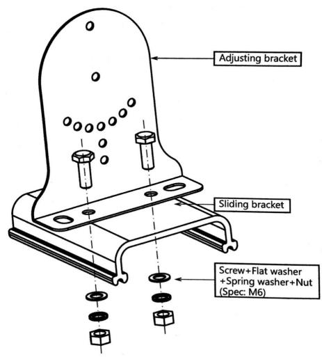
Step 2: Installation of sliding bracket and heater, as arrow points.
