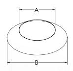
Vent Pipe Collar used to maintain a weather resistant seal between pipe and flashing.
