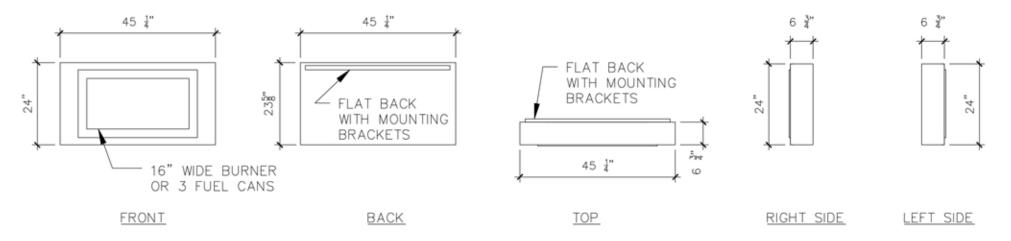
\*Dimensions may vary by 2% (plus or minus) due to material attributes. Template not provided. The Bio Flame recommends using the actual fireplace or burner model when making final cut out.
