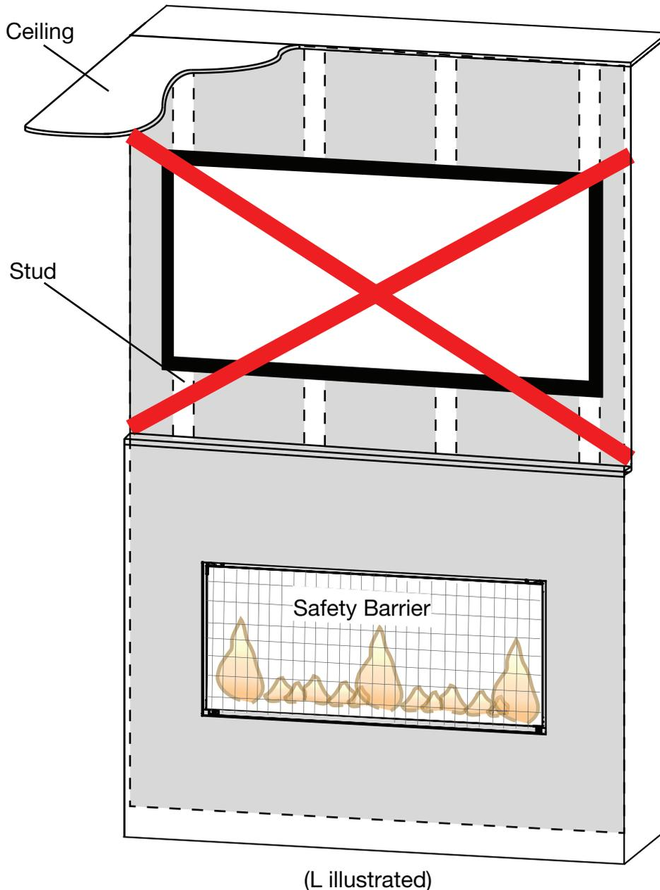
The temperatures above the fireplace for L models will be hot, making it unsuitable for mounting a TV or other objects sensitive to heat above the fireplace without risk of damage.
