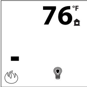
Pressing the light function adjustment button up "**▲**" to single bar will turn on the LED lights. The initiated light colour is white.
