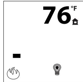
Press the light function adjustment button up "**▲**" to single bar and the LED lights will initiate the rolling colours.
