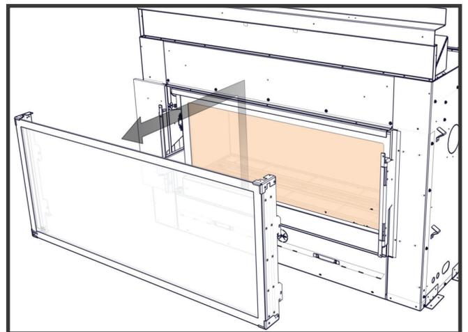
3. Remove the screws and washers securing the GGA-1 to the GGA-1 slider brackets (1 per corner, 4 total).
