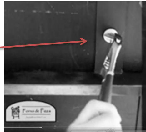
8. Place hearth on top of cart. Tighten 3 underneath screws, then re-install gas regulator (make sure pipe paste or tape for gas is applied on pipe threads).
