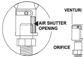
Closing the air shutter will cause a more yellow flame, but can lead to carboning.
