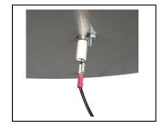
7. Attach the Igniter Spark Probe Wire and the Igniter Ground Wire to the back of the Push Button Assy. Either wire can be placed on either pin.
