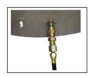
6. Attach the Igniter Spark Probe Wire to the bottom of the Igniter Spark Probe.
