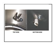
**Tip!** Align one of the burner holes directly underneath the spark igniter probe if possible.
