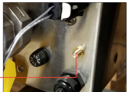
Figure 6.10 – Attach antenna cable
