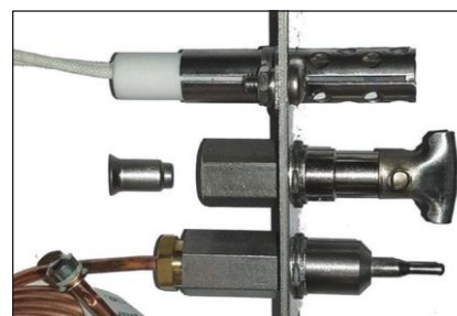
Figure 9.3 – Cleaning pilot orifice
