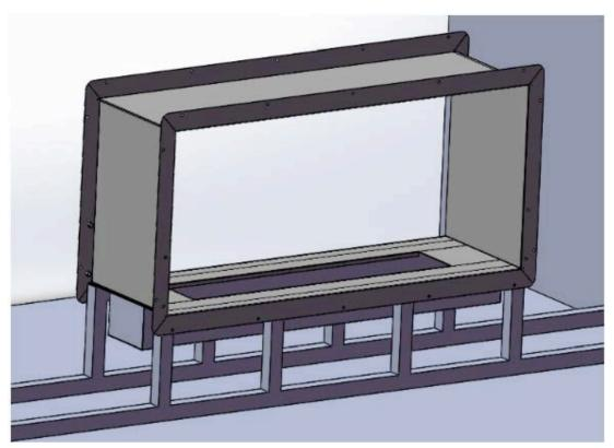
3. Continue building the wall, ensuring that there is a layer of cement board between the stud and your Firebox on all sides.
