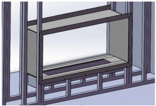
5. Install a stud horizontally on top of the firebox to be able to continue with the wall6.Screw the top of horizontal stud directly to the Firebox brackets (use 0.5 inch metal zips)
