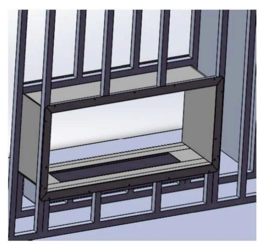
9.Cover the firebox with sheetrock, wonderboard, stones ,etc 10..Mount the glass into firebox
