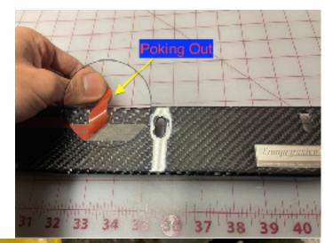
3. <u>Insert</u> Push Pin & <u>adjust</u> side skirt to desire setting.
