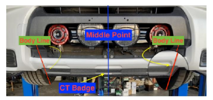
2. After placement confirmation, drill Phillip tap screws (5pc) through the tap screws pits to secure front lip to the bumper.
