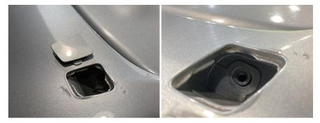
Use a small flat head to open the cover on the top of the stock spoiler. There are two of these, one on each side.
