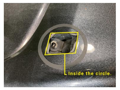
Clean the surface of the stock spolier thoroughly. Remove the liner, and attach the silicone gasket. Make sure the opening is surrounded by the gasket as shown on the left.
