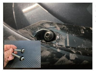
Use the M6 Hex screws and rubber washers included as the replacement of the OEM screws. Tighten it down to complete the install.
