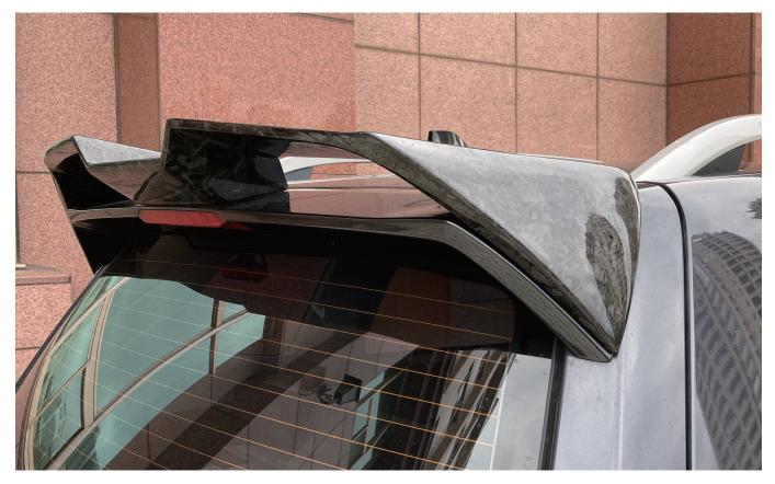
Put the Angel Wing on top of the stock spoiler, align the scewdrive holes properly. NOTE : There are pre-attached silicone gaskets on the Angel Wing as well. It is for the protection of the possible contacting surface of the OEM paint. Do not remove those.
