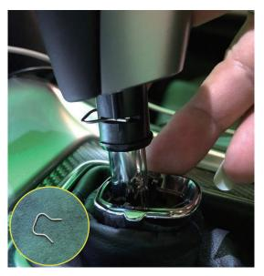
Remove the metal C ring at the buttom of the OE shift knob. Push it forward and it will come off.
