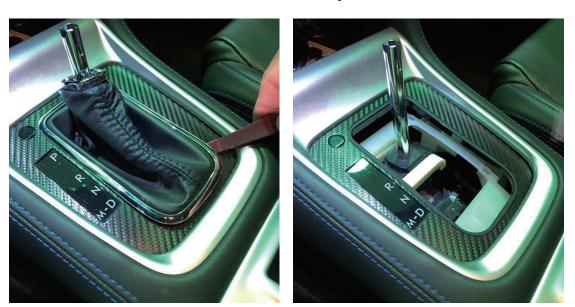
Use the clip removal tool to pop the bottom of the shift boot cover open, and remove the whole assembly.
