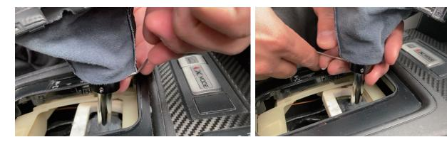
Tighten the three screws with the allen wrench. These three screws are the ones that hold the whole shifter assembly in position.
