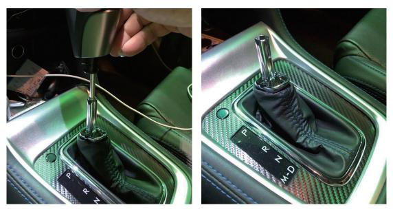
Take out the whole OE shift knob assembly. The next thing is removing the shift boot cover.
