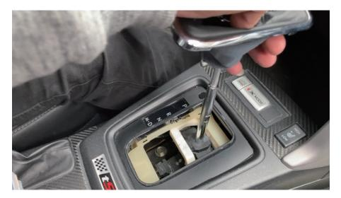
Put the new Shifter kit assembly back in and stop at the depth where the alarm sound stops
