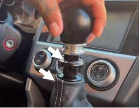
Make some adjustments and make sure the edge of the shift boot is flush, and the Compressive Tuning logo line up with the stitches on the boot.
