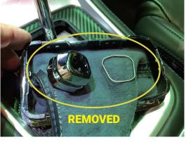
Pull the inside of the shift boot cover out, and remove the metal C ring to seperate the OE shift boot collar from the shit boot cover.
