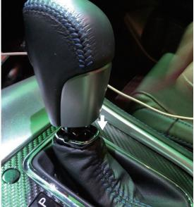
Use the clip removal tool to remove the OEM shifter boot collar.
