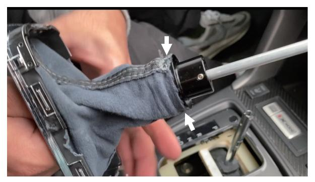
The opening of the shift boot would hold the bottom of the reverse lock piece tight.
