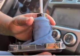
Put the Compressive Tuning Shifter assembly into the shift boot as the orientation shown above and below.
