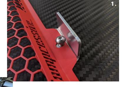
Next, remove the engine cover, and use the built-in bracket on the Air Shields to hook it to upper edge of the inter-cooler.
