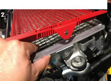
Next, position the bracket to sit under the inter-cooler notch and lined up with the Air Shield hole.
