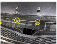
Apply the Clip on the supporting stands. Push the Clip into the hole on the stands.
