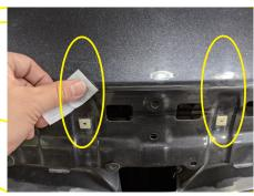
Apply the 3M protecting film to the 2 positions.
