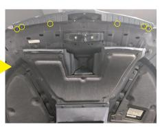
Put the hood bracket and the 4 bolts back on. (Use 8mm wrench)
