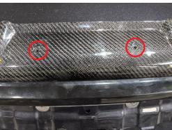
Put the screws on, to hold the bug-shield still. (Not too tight)
