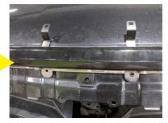
Put the 2 screws of the upper grill frame back, tighten them with the supporting stands beneath it.
