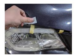
Apply the 3M protecting film to the 4 positions. Then apply the 4 short supporting stands on the same positions.
