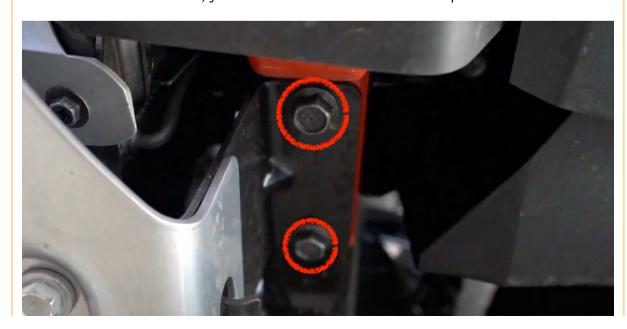
Next using a **10mm Socket** remove the 10mm bolts holding the secondary skid plate to the bumper.
