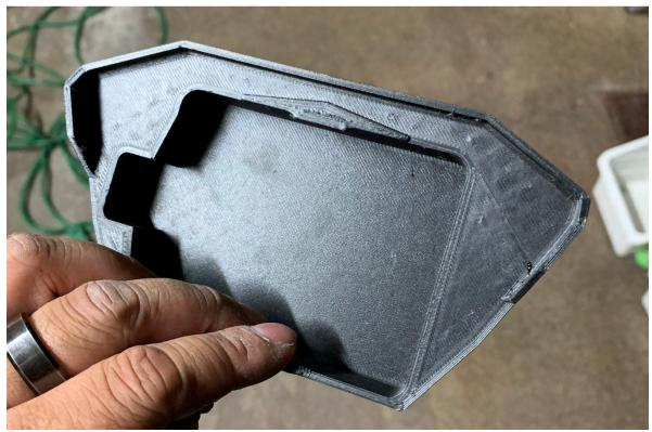
You can now remove the two plastic panel that runs parallel behind the grill. They are being held to the grill with two tabs.
