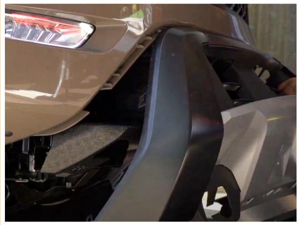
Remove the Styrofoam piece from behind the middle section of the grille. It should just come right off.
