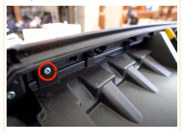
If you have the factory license plate holder then remove them at this point using a **Philips Screwdriver.**
