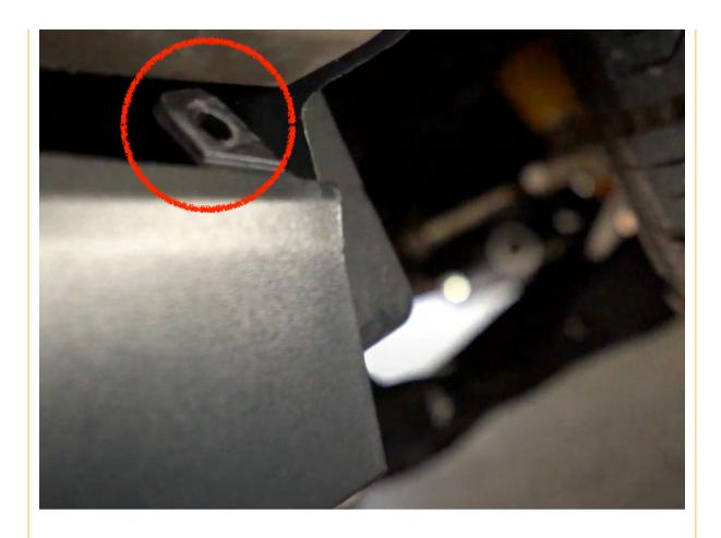
Using a **15mm Socket**, remove the factory skid plates that is attached to the factory tow hooks. There are (2x) on each side. The factory skid plate will fall right off after removing these screws.
