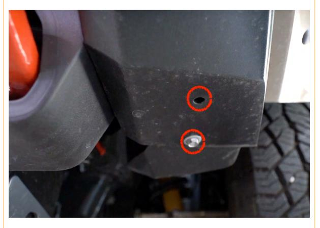
Next remove the 10mm bolts that are hidden behind the plastic lining right behind the factory tow hooks. You'll have to pry the plastic open to get to this bolt. There's two on each side. These 10mm bolts holds the bumper you'll need to remove to the rest of the front bumper.
