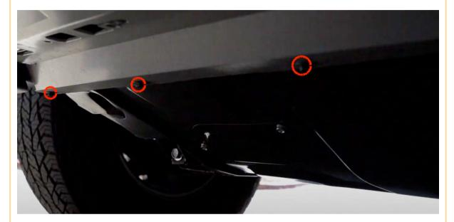
Now it's time to remove that bumper! Being by prying apart each side sections of the bumper. Then pry apart the center section of the bumper. A flat-edged tool will assist in applying the necessary leverage to release the tabs.
