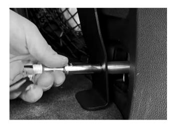
Step 5: Remove slides (C) from package and depress push tab to separate the two halves. Install bolts (F) with Phillips screwdriver into outer frame of the slides loosely. Tighten down once slide frame is properly aligned. Repeat this step for driver and passenger side panels
