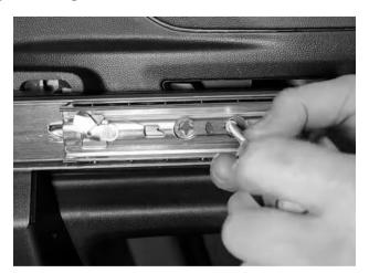
Step 6: Use included hardware (F) to affix inner sleeve of the slides to shelf (A). Please note to keep inner slides pair to the slide frames they were removed from originally.
