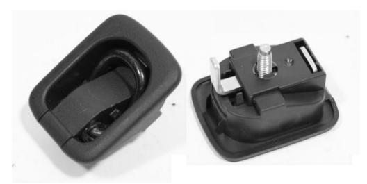
Step 1: Remove Tiedown Caps to access 10mm Bolts (8 in total on both sides). You will be reusing the 6 of 10mm Bolts to install the side molle panels.
