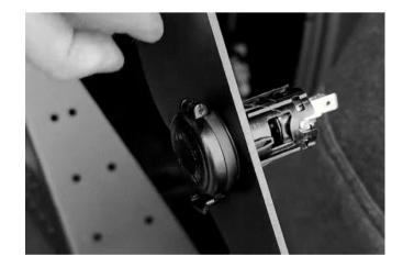
Step 4: Route connector up into the top plastic we removed in Step 3. Repeat Step 1 and install Passenger side panel (B). Reattach 12V connector to socket. Proceed to tighten down all 10mm bolts during this time.
