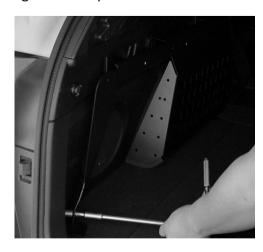
Step 2: Loosely install 10mm bolts top and bottom and side of the driver side molle panel with 10mm socket and ratchet. Longer bolt and spacer (E) will go into bottom leg of driver side panel. When panel is properly aligned, tighten bolts hand tight.
