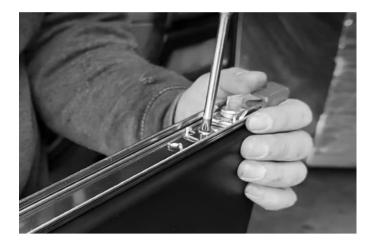
Step 7: This part is preferably performed with the help of another person. Slide shelf (A) with now attached inner slides into the outer frames previously installed on side panels (B). It may be easier to start one side in at an angle like pictured below. Once shelf is properly inserted into the outer slides, push in with even pressure until the shelf locks. Nuts (G) may now also be installed on the inner edges of the shelf for added security.
