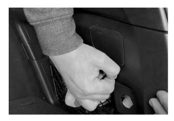
Step 4: Place included O-ring (D) onto 12V power socket and insert into the passenger side shelf support until you hear a satisfying "click". It is important to note the socket is keyed so that it will only fit one way. Do not force this step.
